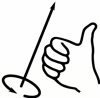
Figure 2.5.2: The right-hand grip rule: curl the fingers of the right hand in the direction of rotation; the thumb points along the angular velocity vector \boldsymbol{\omega} . The same rule determines the direction of angular momentum \mathbf{L} and torque \boldsymbol{\tau} .
